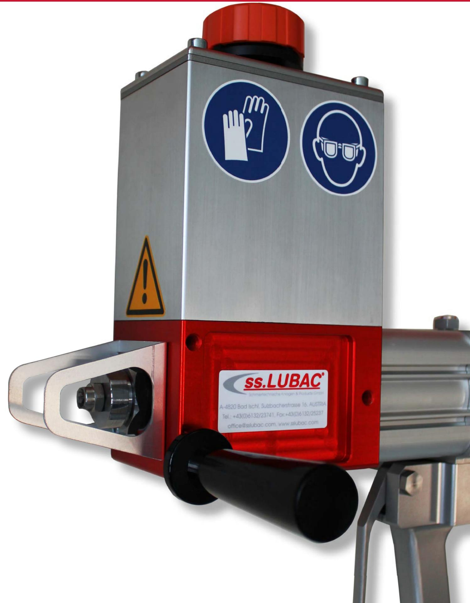
With the portable “**ss.LUBAC RING STAR**” lubrication gun, manually operated with compressed air, lubricant can be introduced or applied directly into the riding ring gap or to the flanks of a rotary kiln. The lubricant is dispensed from safe distance by means of a “spray process” and is applied precisely to the target surface. The gun is connected to the compressed air supply network at the operating site by means of a compressed air quick coupling.
