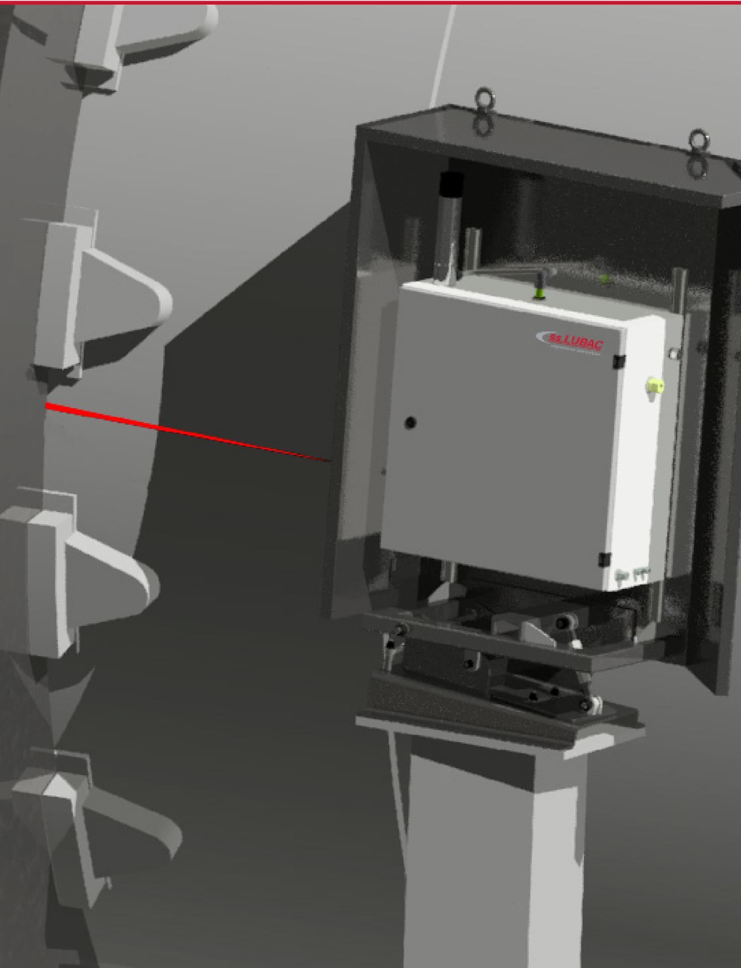
▶ The “**ss.LUBAC RING STAR Automatic**” application unit is set up within a stainless sheet steel safety cabinet. An automatic “**ss.LUBAC RING STAR**” lubrication gun is built into the cabinet.
